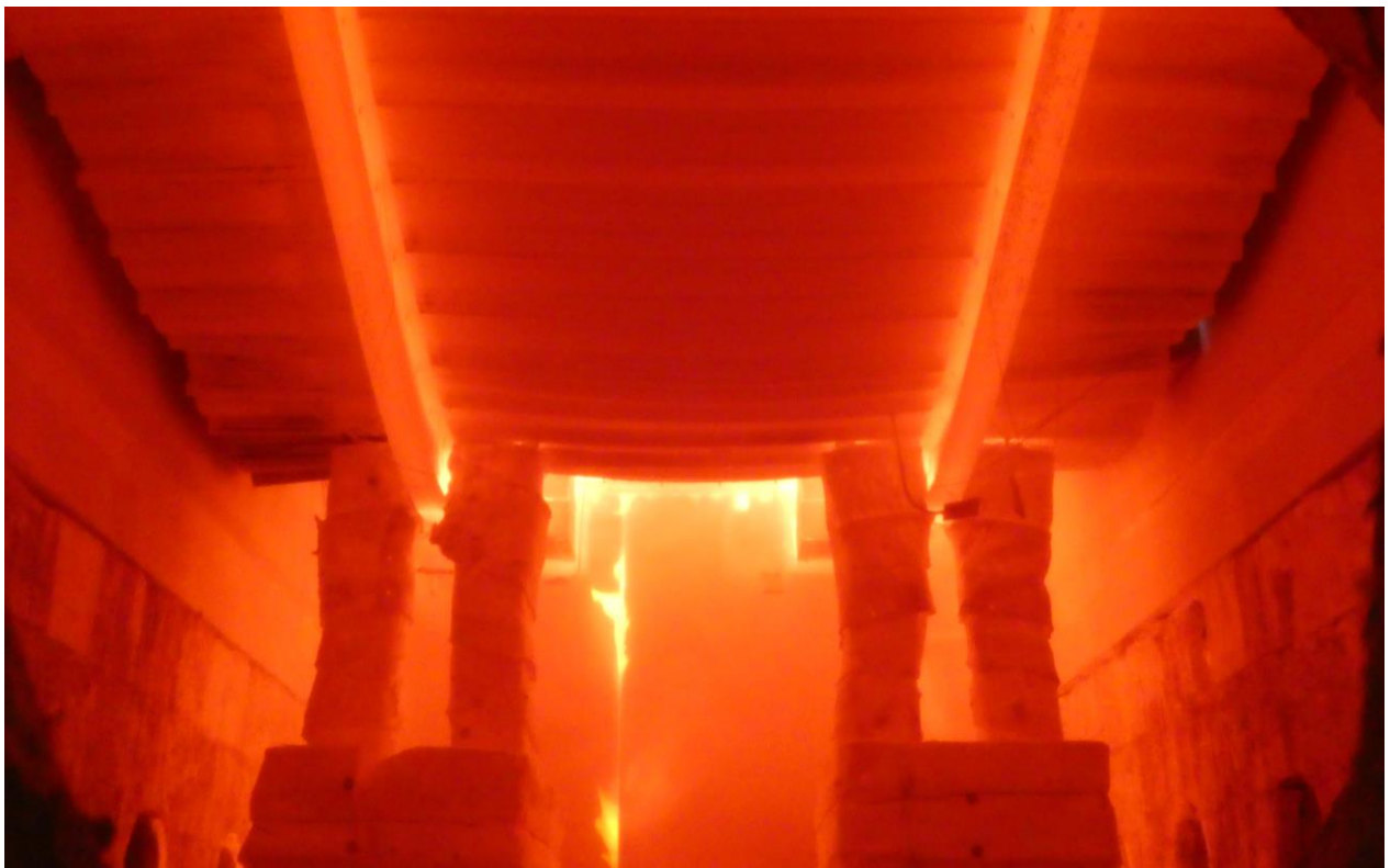
EF after 80 minutes of the test and turn off the burners
