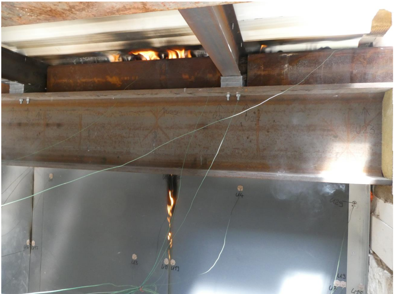
Ignition of the cotton pad and sustained flaming in 58 th minute of the test
